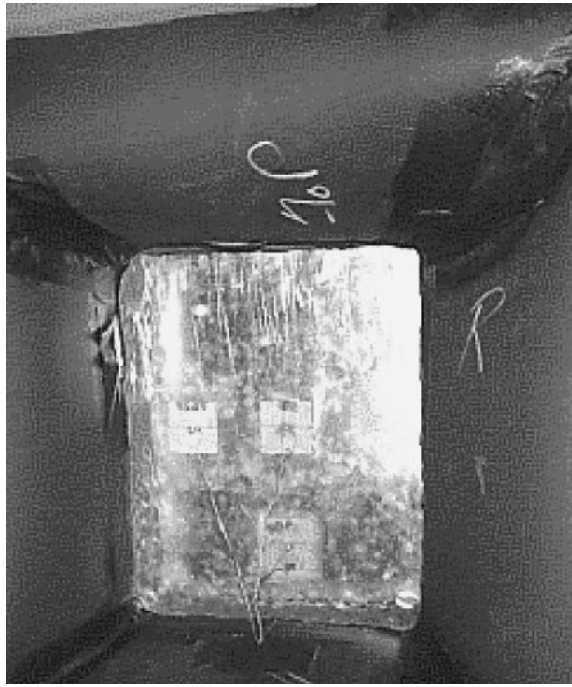
Figure 5. Plate with electrically shunted PZTs in the (reception chamber side) modified test window of the transmission loss facility.
